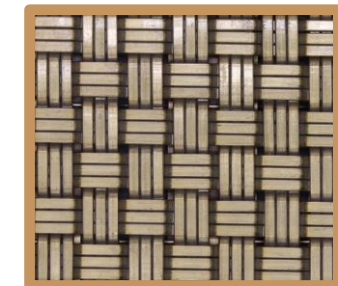
QKCWM-07 Warp Diameter: 0.75x2mm Weft Diameter: 0.75x2mm Warp Pitch: 15mm Weft Pitch: 15mm Weight: 6.5kg/m 2 Opening Area: 9.2%
