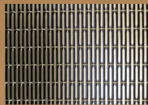
QKCWM-01 Warp Diameter:1.5mm Weft Diameter:2mm Warp Pitch:4mm Weft Pitch:17.5mm Weight:2.5kg/m2 Opening Area:45.7%
